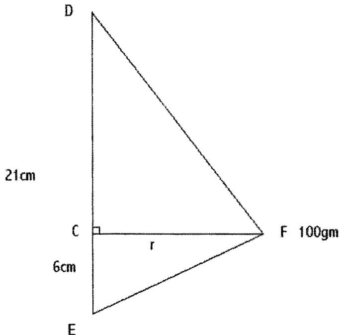
A light inelastic string of length 27cm is attached to two points D and E on the vertical shaft DE, distance 21cm apart, E being vertically below D. F is a smooth ring of mass 100gms threaded on the string. The system is such that F moves with constant speed in a horizontal circle 6cm above E.
